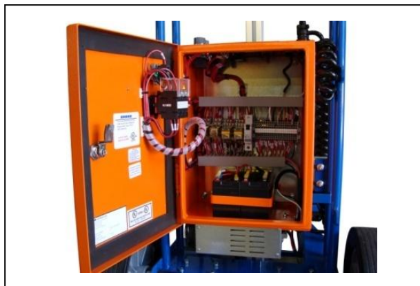
Figure 1.4 – Control Cabinet, Internal
